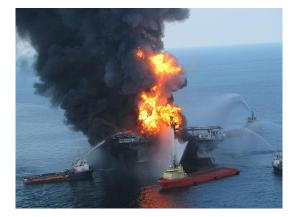
No one could have known that later that same day, the entire rig would go up in flames due to a malfunction in the rig's blowout preventer. Around ten o'clock that evening the oil rig became a fireball. Gigantic flames shot straight up in the air. The crew scrambled to board the rig's life boats and escape to safety. Sadly, eleven members did not survive.
